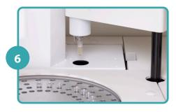
Luminescence reading directly in the cuvette
