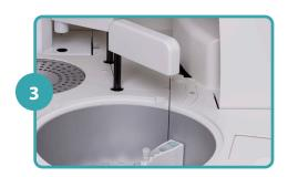
Pipetting needle washing with decontamination reagent
