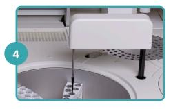
Disposable tips and cuvettes to avoid sample carry-over
